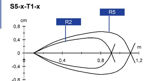
The detection diagrams indicate the typical operating distance with excess gain 1.
